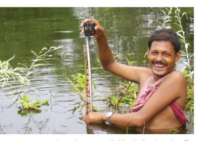
measuring poles were provided by the Darwin project. The water level records will give us information about the degree of availability of water all year round in the fish ponds. The source of water in the fish ponds is most important for the good fish production. These data will be used for the fisheries management plan.
